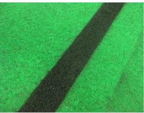
Lines should give an EV3 Reflected Light Reading of 0
