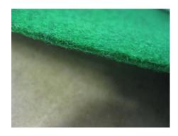
Short Fibre, Thickness 3-5 mm, EV3 reflected light reading 3 or above
